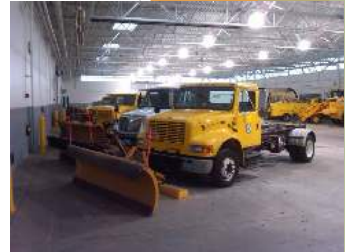
Parking stalls sized to store plows
